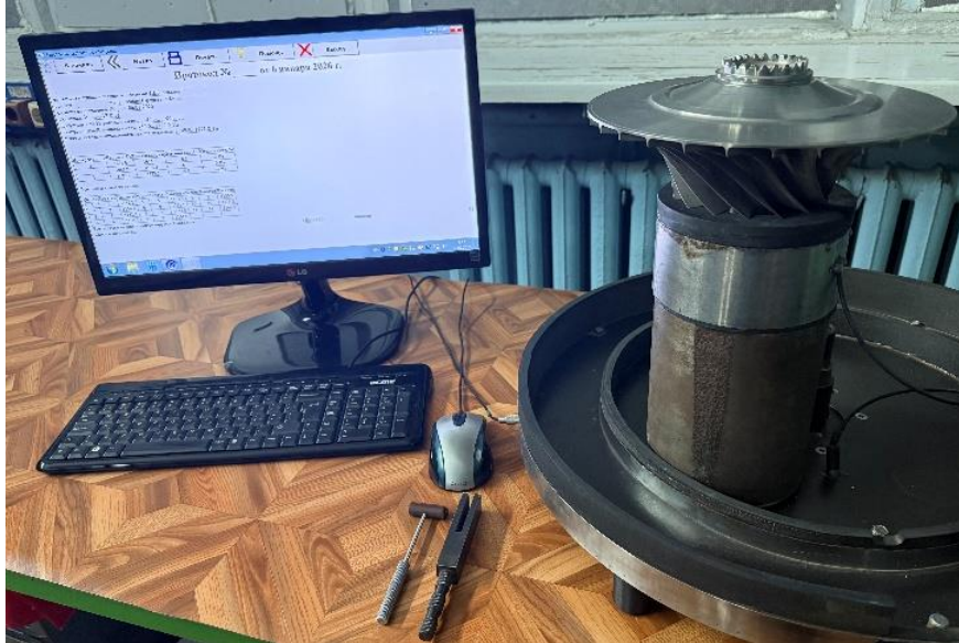
Figure 1. «MIKAT-ChKM» unit for automatic frequency inspection.
