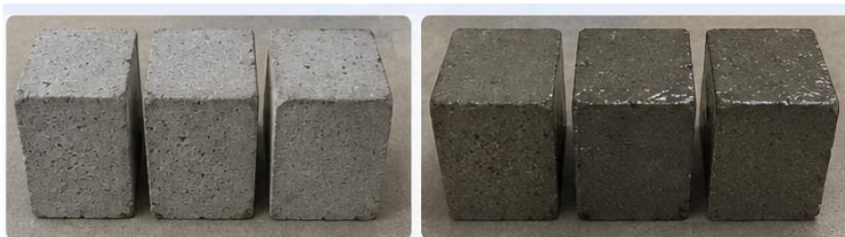
Figure 1. Concrete specimens for testing without treatment and with polymer impregnation.
