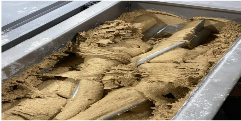
Figure 3. Dough kneading in the final kneading chamber
