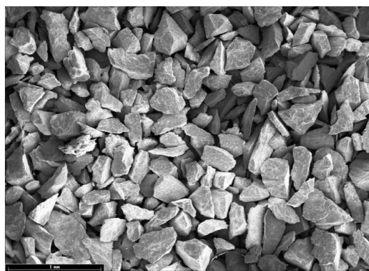
Figure 3. Solder powder 18XFC (Sizes of powder parts from 0.1...0.5 mm)
