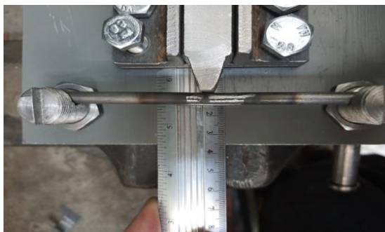
Figure 5 a) Determination of the bending (initial position of the sample)
