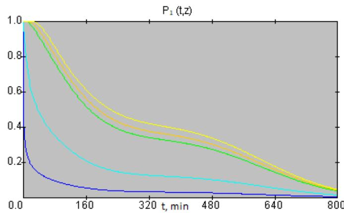
**Figure 2.** Pressure profile evolution in macropores at time for various locations at a heterogeneous media  $Z=1.0$  (yellow),  $Z=0.7$  (orange),  $Z=0.6$  (green),  $Z=0.2$  (cyan),  $Z=0.05$  (blue)
