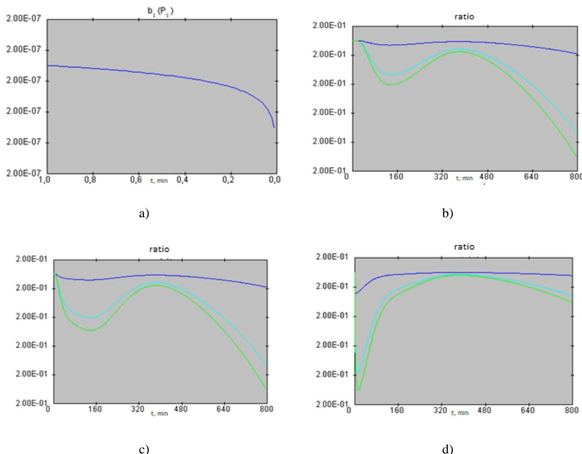
**Figure 4.** Consolidation coefficients a) - Dependence of the nonlinear consolidation coefficient on the pressure value, b), c), d) - Ratio of nonlinear consolidation coefficients in the interparticle and intraparticle spaces b)  $Z=1$ , c)  $Z=0.5$ , d)  $Z=0.05$ ,  $X=0.95$  (blue),  $X=0.5$  (cyan),  $X=0.05$  (green)
