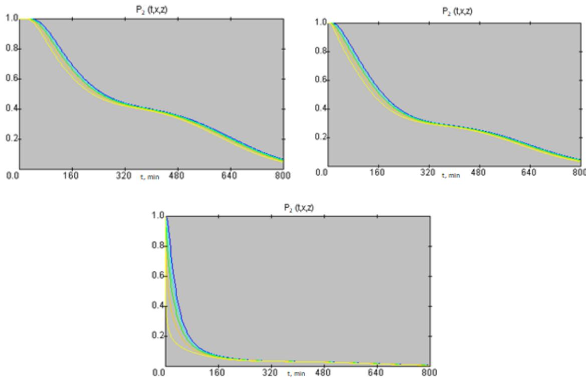
**Figure 3.** Pressure profile evolution in micropores at time for various position of the particle in the medium: a)  $Z=1$ ; b)  $Z=0.5$ ; c)  $Z=0.05$ ;  $X=1$  (yellow),  $X=0.8$  (orange),  $X=0.6$  (green),  $X=0.4$  (cyan),  $X=0.05$  (blue)
