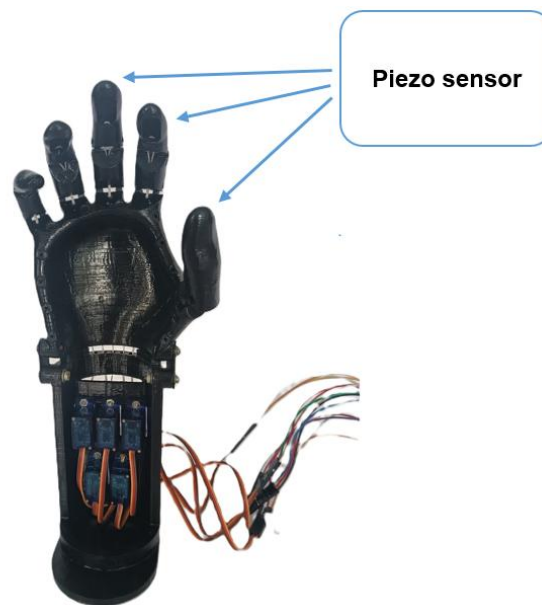
Figure 1: Scheme of placement of piezo transducers in the manipulator robotic arm
