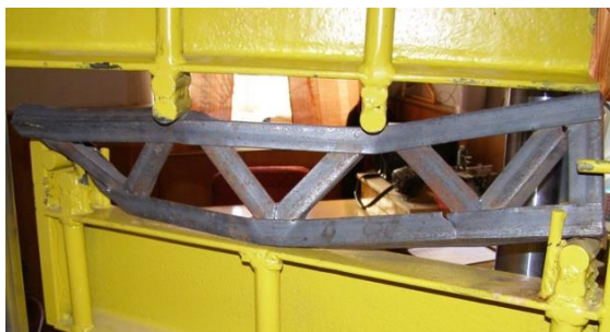
Figure 8. Physical model after fatigue failure
