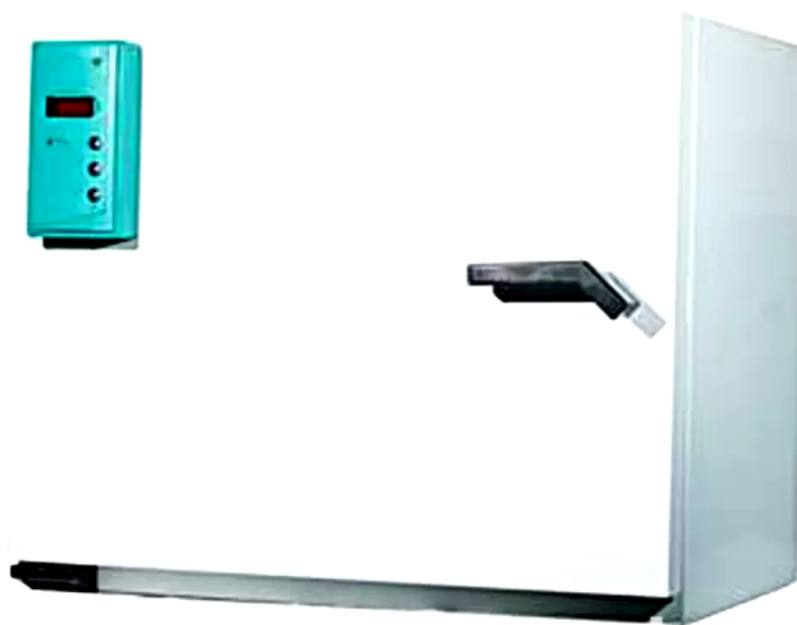
Figure 1.4 – ShS-80 N dry-air thermostat
