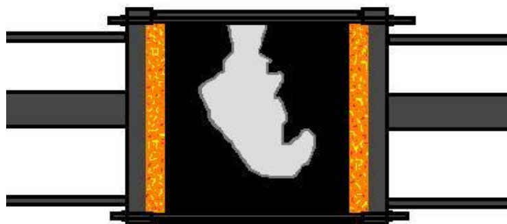
Figure 77 – Mold for slush casting gross sectional view of inside of casting a certain amount of time ( T_1 ) after pouring
