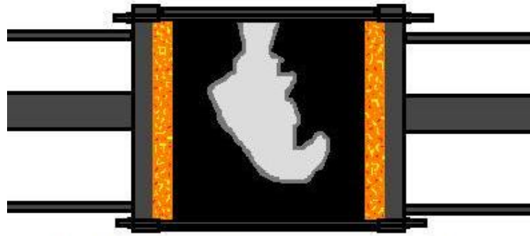
Figure 78 – Mold for slush casting gross sectional view of inside of casting a certain amount of time ( T_2 ) after pouring also note ( T_2 > T_1 )
