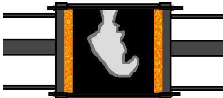
Figure 79 – Mold for slush casting gross sectional view of inside of casting a certain amount of time ( T_3 ) after pouring also note ( T_3 > T_2 )
