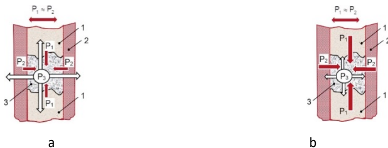
Fig.1 Formation schemes of a) positive flux for P_3 > P_1 \approx P_2 and b) negative flux for P_3 < P_1 \approx P_2 , where: 1 - bone tissue; 2 - soft tissues of the body; P_1 , P_2 – radiation power per unit area of bone and soft tissues of the body; P_3 – radiation power per unit area of the implanted material.
