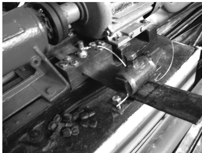
Fig. 6 Appearance of the plate DVA under study
