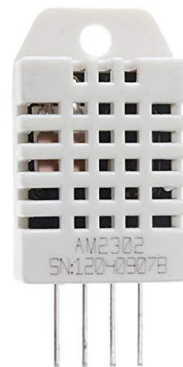
Figure 3.1 - Humidity and temperature sensor DHT22.
