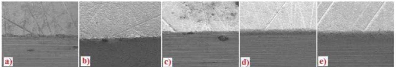
Fig. 2.8 - Cutting edge received by: a) grinding, b) laser treatment to edge radius 5 \mu\text{m} , c) 5 \mu\text{m} , d) 10 \mu\text{m} , e) 15 \mu\text{m} [10]
