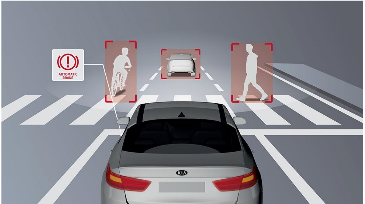
Fig. 1.2. Automatic brake system from KIA Motors [5]
