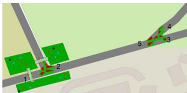
Figure 4. The location of queue counters: 1 – ramp from Bykova street to intersection; 2 – ramp from the bridge to Bykova street; 3 – straight traffic towards Symonova street; 4 – left turn ramp from the bridge; 5 – ramp from the Bypass to the bridge.
