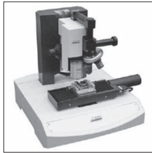
Figure 6 CSM Microhardness tester device used for measurements of micromechanical properties
