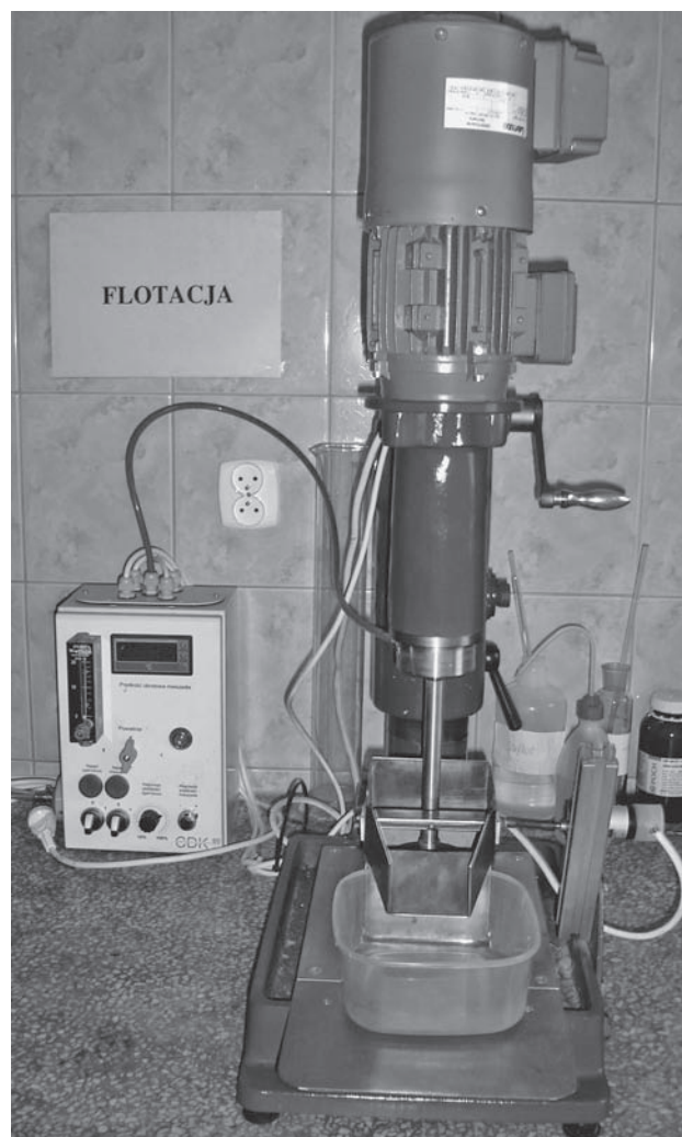
Figure 1 Laboratory-scale flotation process equipment [1].
