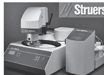
Figure 4 Struers Tegra Pol 35 device for sample grinding and polishing
