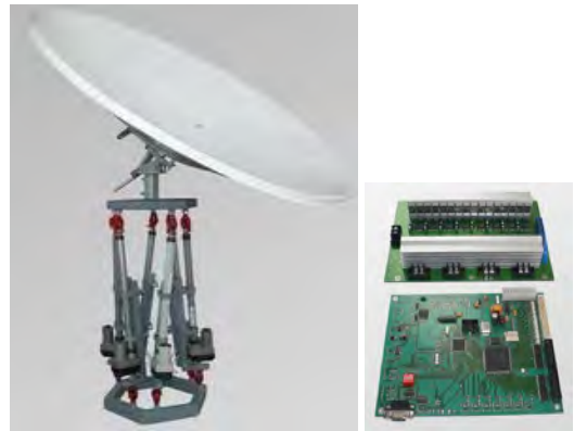
Fig.1 AS prototype with RSD of the Stewart platform (Hexapod) based, and the control unit.
