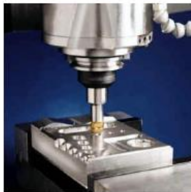
Fig.5.20. End milling operation used to cut a pocket in an aluminum workpart.
