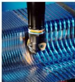
Fig. 5.23. Close-up view of a hemispherical ball-end mill with indexed carbide inserts used for rough cutting of a three-dimensional surface.
