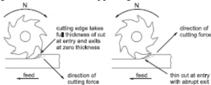
Fig. 5.15. Two types of peripheral milling.
