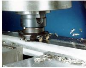
Fig.5.19. Conventional face milling operation. The face-milling cutter machines the entire surface. The cutter diameter is greater than the workpart width.
