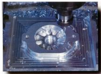
Fig. 5.24. Surface contouring of die cavity. The cutter used is a high-speed steel ball-end mill.
