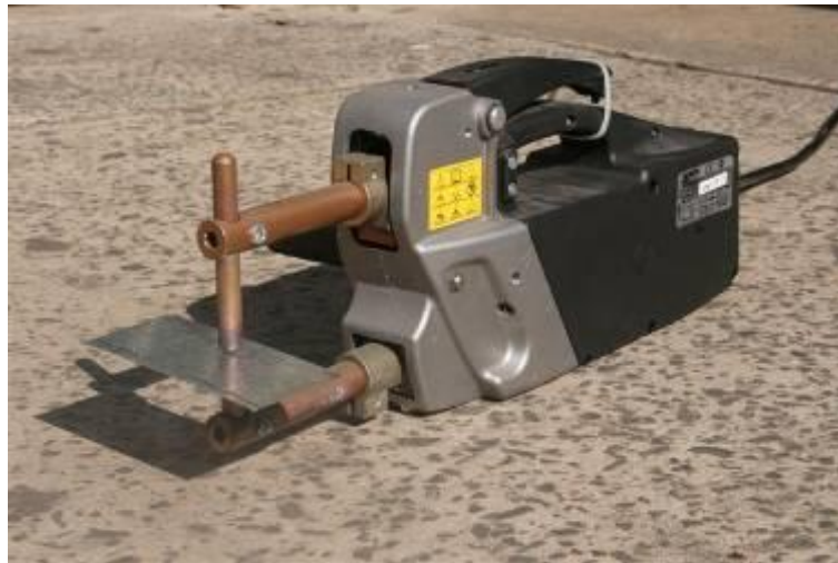
Fig 4.16. A spot welding unit with sheet metal in place
