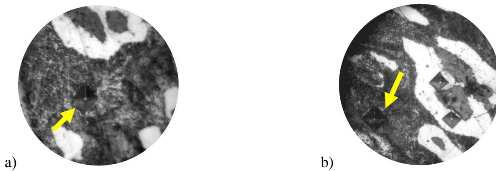
Figure 8. Cast iron structure BЧ50 (x380): a) in initial state; b) after deformation
