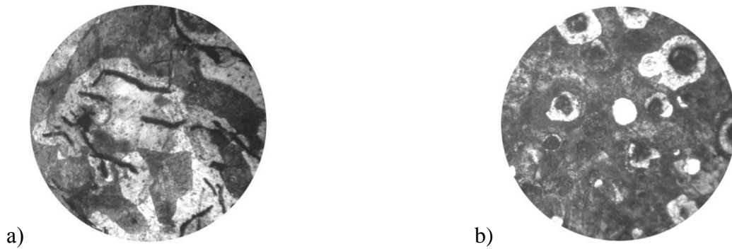
Figure 6. Microstructure of samples (x380): a) CЧ20; b) ВЧ50
