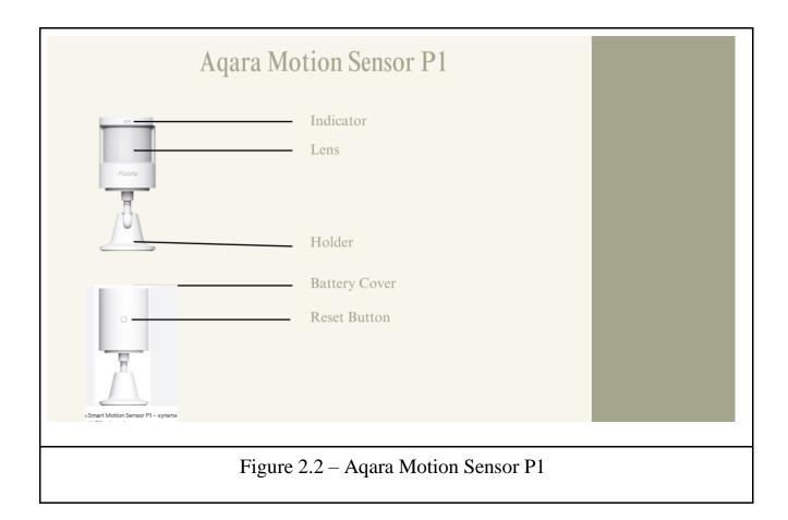
Description: Detects movement of a person or an object. This is basically connected to the light and also the placement of the Aqara motion P3 sensor, should not be far from the light. This sensor is either placed on the wall or on a flat surface area for better communication with the lighting system. It also can be connected to mobile wifi or home wifi for an effective process.
