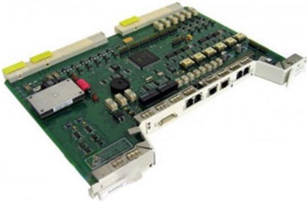
Figure 3.9. AIC-I – alarm controller card
