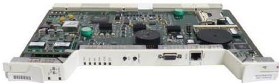
Figure 3.7. TCC2 – card of synchronization, communications and control
