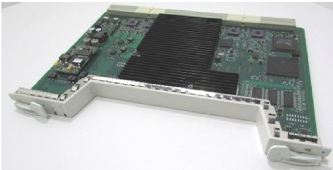
Figure 3.10. XC-VXC-10G – Optical switching module
