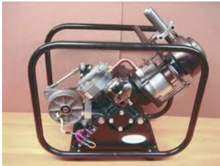
Fig. 1.13 Industrial Stirling engine with a capacity of 1 kW
