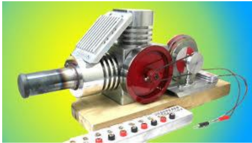
Fig. 1.12 Modern Stirling engine with electric generator
