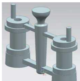
Figure 1 – 3D model of the gating-feeding system
