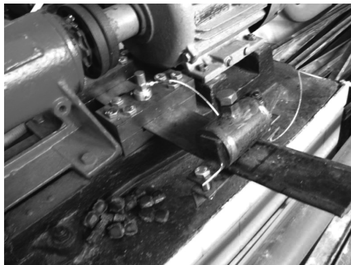
Fig. 6 Appearance of the plate DVA under study
