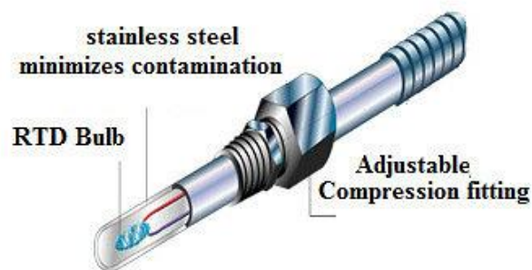
Figure 2.4. Resistor Temperature Detector (RTD)
