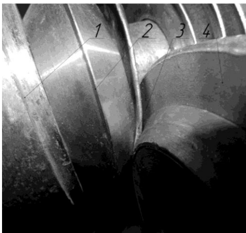
Figure 7. WSCP manufacturing with shaping tool: 1 – mandrel; 2 – bushing; 3 – curved profile; 4 – roller
