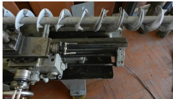
Figure 3. WSCP manufacturing with screw mandrel
