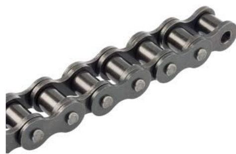
Figure 2. Link plates with curved side edges („figure-eight“ type) – in most drive chains (classical shape)
