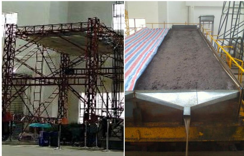
**Fig. 2 - Artificial simulated rainfall device**
