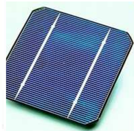
A solar cell made from a monocrystalline silicon wafer
