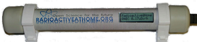
Fig. 1. Dedicated hardware sensor Radioactive@Home.
