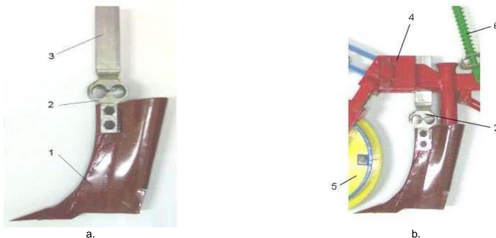
Fig. 8 - Tensometric ring device for determining the forces in fixing arm of soil opener (share) [1, 2]: a- mounting the tensometric ring at the soil opener; b- soil opener mounting on the body of the sowing section; 1-soil opener; 2-tensometric ring; 3-fixing arm devices;4- body of sowing section; 5- cutter disc; 6-spring of section
