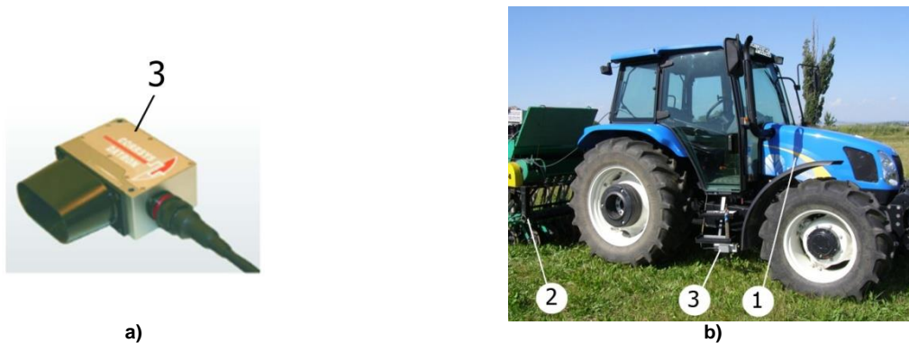
Fig. 12 - Optical speed transducers AQUA L 350 type (a) and transducer location on the tractor (b) [1]: 1-tractor 4 WD (100 HP); 2-oversowing machine (type) MSPD-2,5; 3-optical transducers of speed
