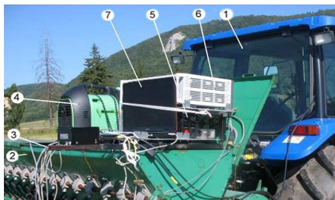
Fig. 13 - Location of measurement and data recording equipment on the tractor-agricultural machine system: 1-tractor; 2-grassland oversowing machine; 3-frame for placement of measurement and data acquisition equipment; 4-power supply; 5- voltage stabilizer; 6- booster modular system (MGCplus); 7-laptop P4
