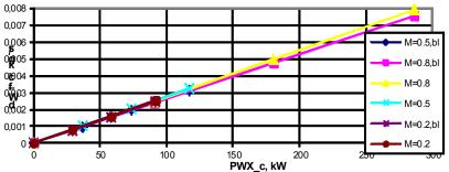
Figure 2. Relation between mechanical power off take and incremental fuel flow (booth corrected for sea level standard conditions) at different Mach numbers, with and without air bleed
