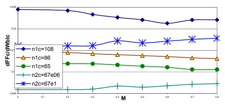
Figure 3. Relation between the derivative dFFc/dWblc and the Mach number, at different engine fan rotational speeds in percents and different points of air bleed
